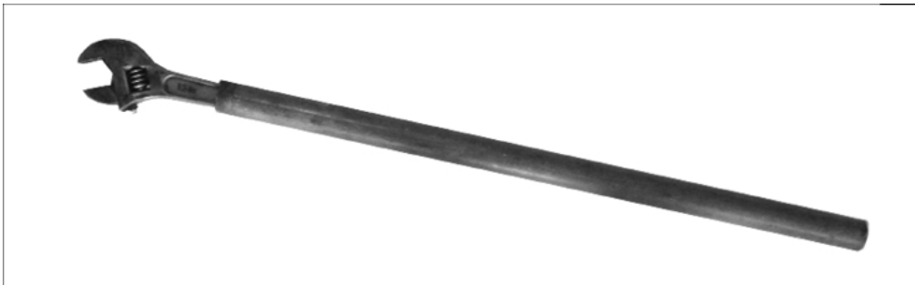
A simple pipe to be used as a cheater, shown here applied to a large wrench.
